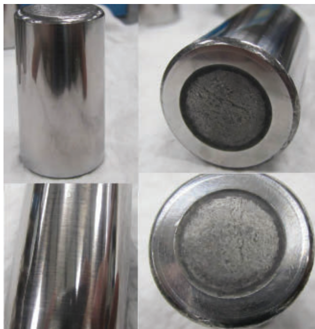
A 216-hr run left the raceways (left) and the roller elements of the bearings within the customer's requirements. (Fig. 6).
