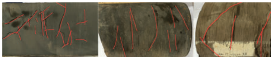
Red lines drawn on cores show the distribution and width of natural fractures (Fig. 2).
