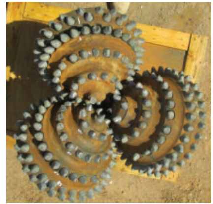
This TCI bit was brought to the surface after 216-hr run because of a suspected washout in the drilling string. The bit was dull-graded (Fig. 5).
